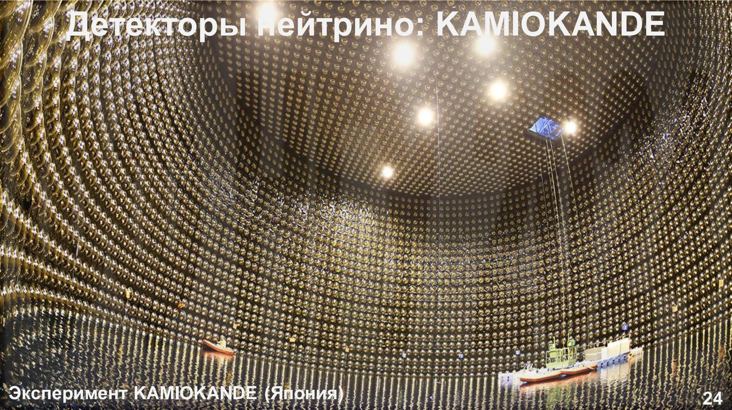
The image shows the interior of the Kamiokande neutrino detector, a large cylindrical cavern. The walls and ceiling are covered in a dense grid of photomultiplier tubes (PMTs), which appear as a shimmering, textured surface. Several bright lights are visible on the ceiling, and a blue object is suspended from the ceiling by ropes. In the foreground, a small boat is visible on the water surface, and another larger boat is on the right side. The overall atmosphere is dark and industrial.
