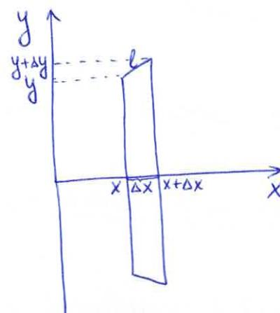
$$\Delta S = \pi(y + y + \Delta y)l = \pi(2y + \Delta y)\sqrt{(\Delta x)^2 + (\Delta y)^2} = \pi(2y + \Delta y)\sqrt{1 + \left(\frac{\Delta y}{\Delta x}\right)^2} \Delta x$$
