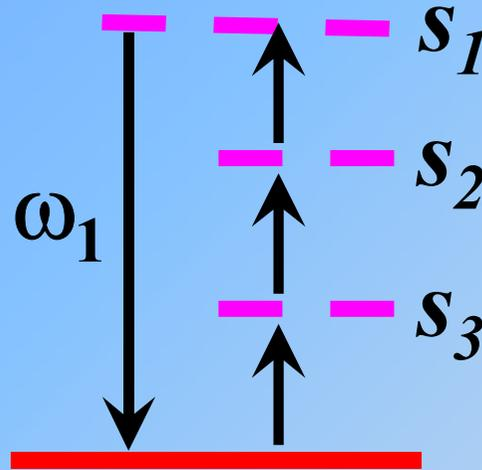
$$V_{fi} = \sum \frac{V_{fs_1} V_{s_1s_2} V_{s_2s_3} V_{s_3i}}{(E_i - E_{s_1})(E_i - E_{s_2})(E_i - E_{s_3})}$$
