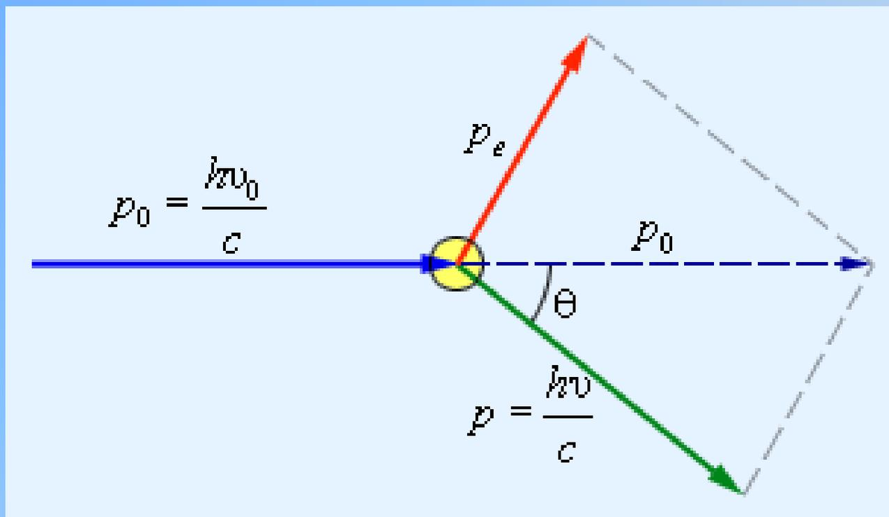
$$\hbar\omega + mc^2 = \hbar\omega' + \sqrt{p_e^2 c^2 + m^2 c^4}$$
