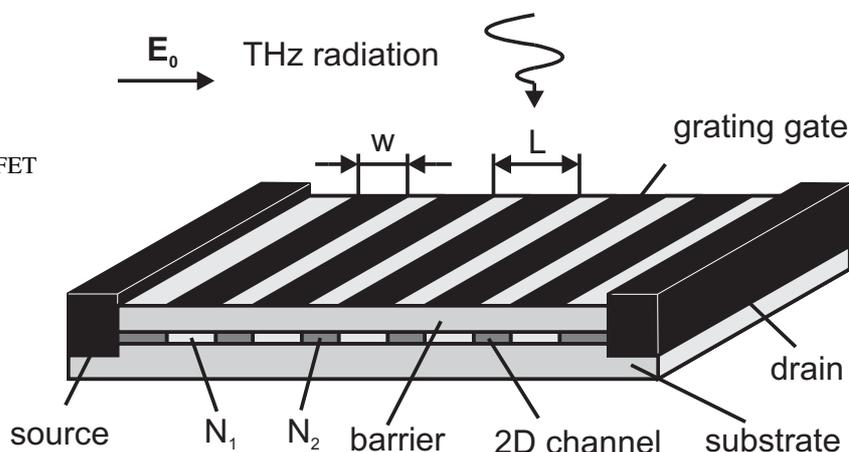
Fig. 2. Schematic view of the FET structure with a grating gate
