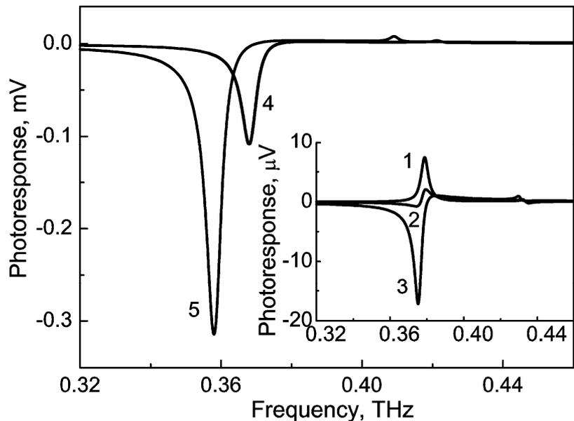
Fig. 4. Photoresponse vs frequency near the fundamental plasmon resonance for a density modulated grating-gated GaAs/AlGaAs FET structure at different values of the modulation factor  $\alpha$  (see text):  $\alpha=0$  (curve 1),  $\alpha=0.003$  (curve 2),  $\alpha=0.01$  (curve 3),  $\alpha=0.05$  (curve 4), and  $\alpha=0.1$  (curve 5) [15]
