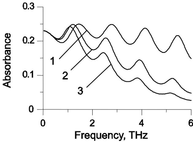
Fig. 3. Calculated absorption spectra of AlGaIn/GaN grating-gate FET structure with 1- $\mu\text{m}$ -wide grating-gate fingers for three different slit widths: 0.1  $\mu\text{m}$  (curve 1), 0.3  $\mu\text{m}$  (curve 2) and 0.5  $\mu\text{m}$  (curve 3) at room temperature [14]
